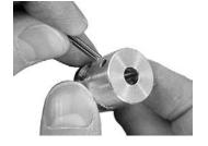
I. Insert the 3mm spring pin partially into the coupling. Insertion may be easier by first squeezing the tip slightly with pliers.
